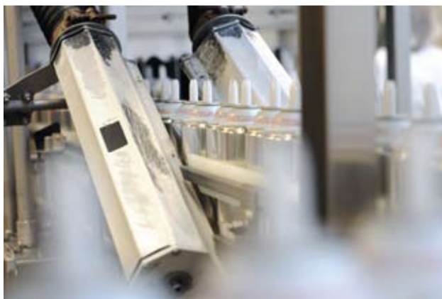
After each aerosol can is rinsed, an Admark dryer supplied by RE Morrison blow dries the can to allow a proper label application seal.
