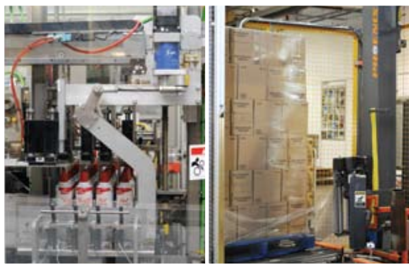
A Douglas Machine case packer uses ELAU servo motors to package product into corrugated cartons.
