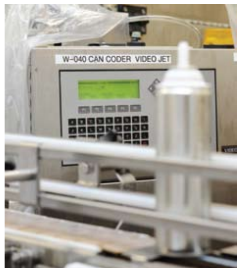
Utilizing military time, a Videojet Excel inkjet coder applies best before date and time of packaging information to each aerosol can.
