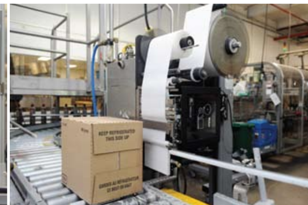
Manufactured by Weber Marking Systems, a labeler applies a pressure-sensitive label to cartons of aerosol whipped products at Gay Lea's main Guelph facility.
