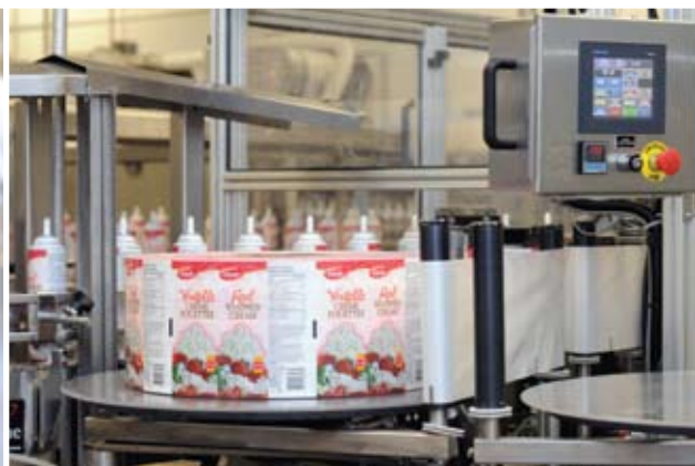
Utilizing a Schneider Electric Telemecanique Magelis viewscreen, an Associated Packaging system wraps labels around cans of Gay Lea Real Whipped Cream.
