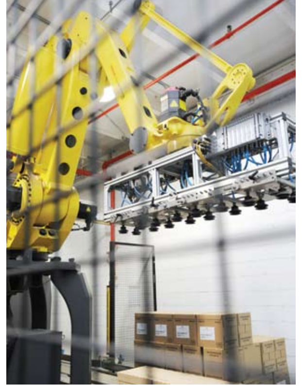
Cartons of product are directed toward a FANUC Robotics M-410iB 160 robotic palletizer.
