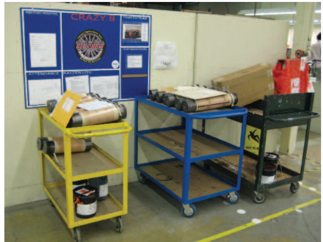
Labelad logs its Kaizen events on bulletin boards throughout the plant. Also, supplies and job orders are self-contained on carts.
